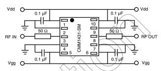
Note: Due to the high gain of this device it is highly recommended to maintain the reverse isolation (S12) above 50 dB.
